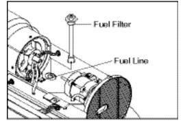
Figure 18. Removing Fuel Filter
